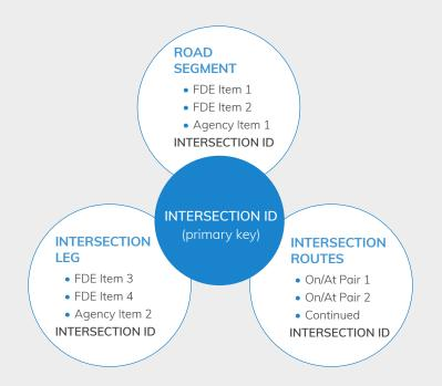
Using that single-point location and a primary key, the other key attributes needed to support the intersection MIRE data structures can be associated to the intersection.
